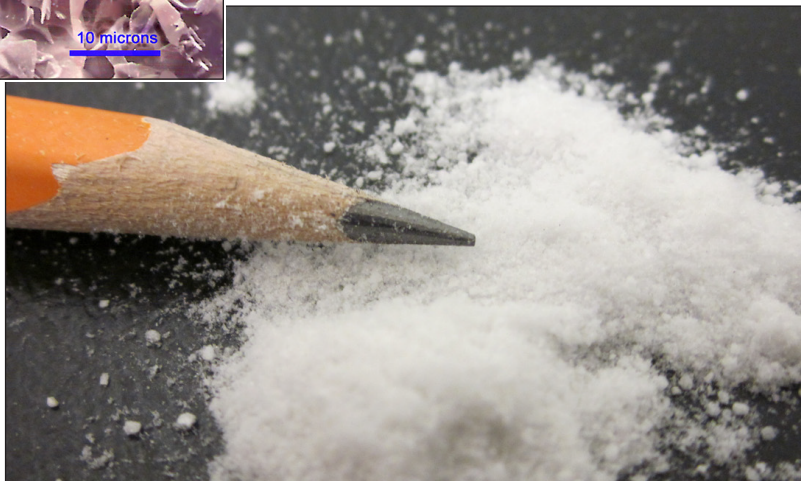
A filter aid is a finely graded material which, when added to the liquid to be filtered, collects on the septum (a screen or cloth). The filter aid forms a porous layer on the septum and thus the filter aid is the filtering medium that traps the solids being removed and prevents them from blinding the septum.
